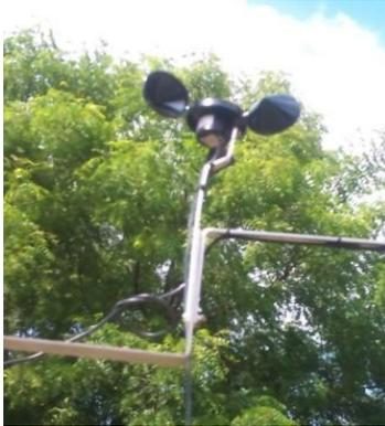
An **anemometer** is a device for measuring wind speed, and is a common weather station instrument. It measures the horizontal wind speed. Cup type anemometers are the general standard type of anemometer. It consists of three hemispherical cups which are mounted at equal angles to each other on a vertical shaft. They are robust and resistant to turbulence and skew winds caused by masts and traverses.
