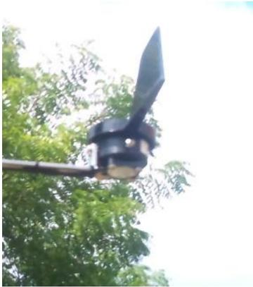
The wind direction sensor is a sensitive wind direction indicator that provides azimuth data as indication of wind direction. A Hall Effect angular position sensor is used for accurate position measurement of the wind direction vane. This provides full 360 degree detection. Utilizing Hall Effect detection technology makes the sensor more sensitive, accurate, with a higher resolution, while significantly enhancing the reliability and durability of the sensor.
